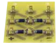
9879810 Rectifier, Full Wave Bridge, Single-Phase, 300V, 3A
