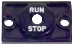
32554 Bezel, Run/Stop Keyswitch, 1.56"H x 2.44"W, 1/4" dia.; mounting holes on 2" centers
