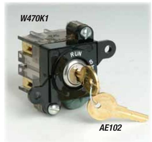
WESTINGHOUSE TYPE "E" KEYED STOP SWITCH ASME A17.1, 210.2(v), 1990 requires keyed stop switches in new passenger elevators where STOP switches are specified. Our Westinghouse complete keyed switch meets this requirement with great attention to detail.
