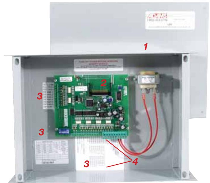
1. Solid box construction and powder-coat finish protect sensitive electronics
