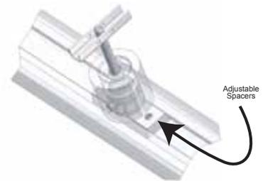
Exterior Cab Mounting Spacer
