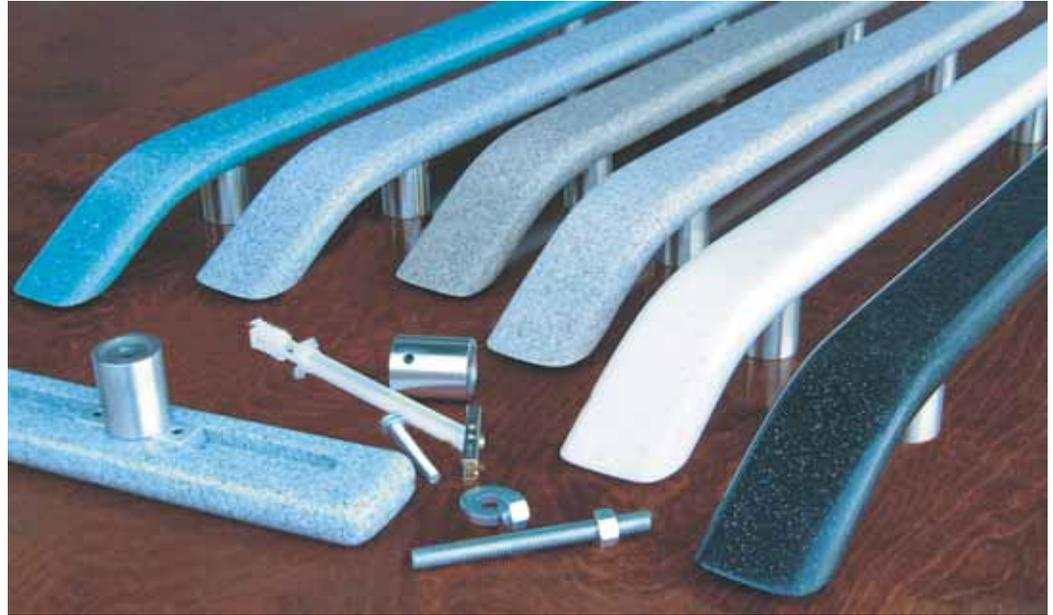
**Designer Series:** Constructed from Solid Surface, (mineral-filled acrylic polymer) materials, in a variety of sandstone colors. The one piece channeled design of these handrails allows for easily adjustable spacer locations that can be slid along the length of the handrail and locked into place. Manufactured directly from your measurements and specifications on our easy-to-use worksheet, our accuracy matches your measurements and your standards. Meets ADA requirements.
