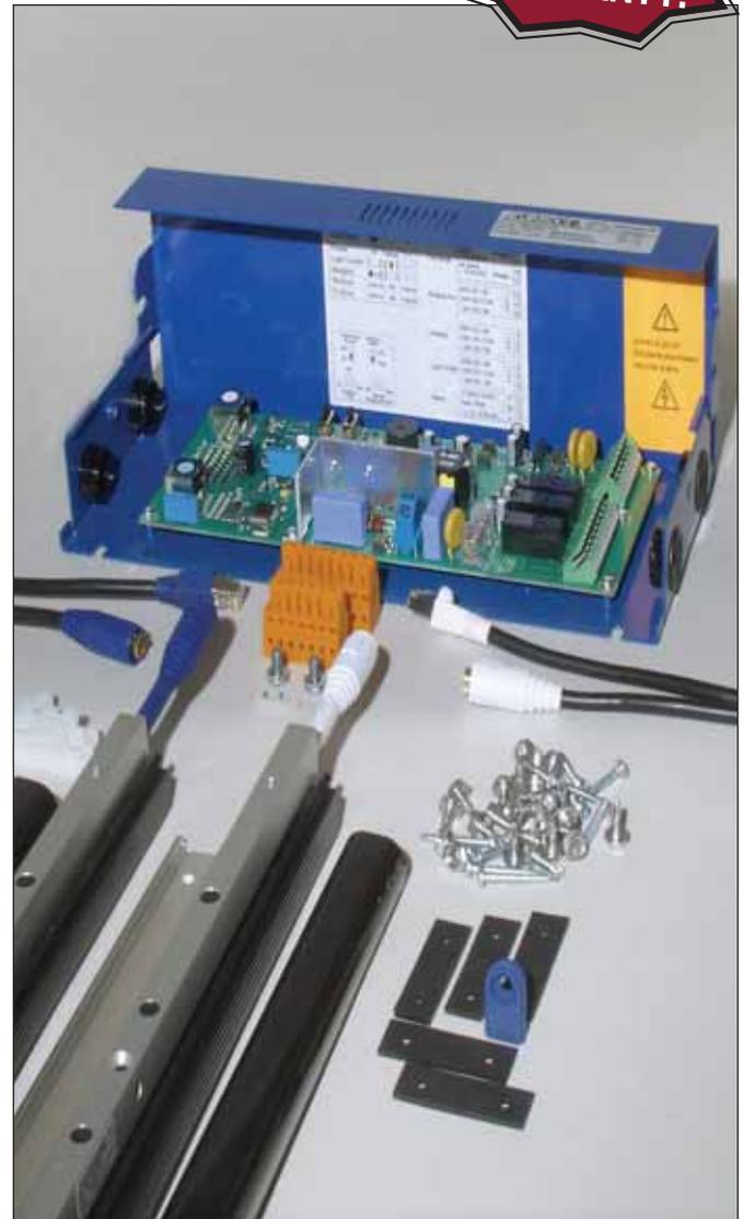
***Built-in nudging helps keep elevators moving in environments where riders are likely to hold open the doors. Nudging time is adjustable from 1-60 seconds***
