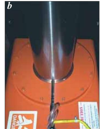
*LifeJacket's arms remain open during normal elevator operation (a). When the unit senses uncontrolled downward movement, the arms close immediately (b)—bringing the elevator and its passengers to a soft and safe stop*
