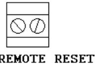
Connecting a normally open switch or contact to this terminal will allow the latching alarm contact to be reset remotely. Activating a switch or contact connected to this terminal will have exactly the same effect as pressing the relay contact– **RESET** button. The switch or contact used should be rated to switch a 100mA load @ 12VDC.
